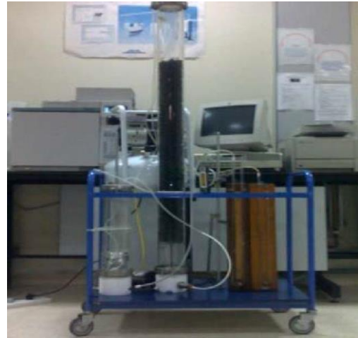
Figure 1. Pilot Plant Scale Biofiltration Equipment. Source: Shareefdeen et al. , (2011)
