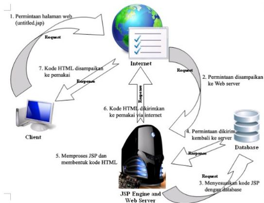
Gambar 1. Servlet/ JSP Application Architecture (Dihin, 2009)
