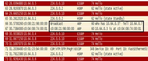
Figure 4. Star ARP Capture Packet Frames in HSRP
